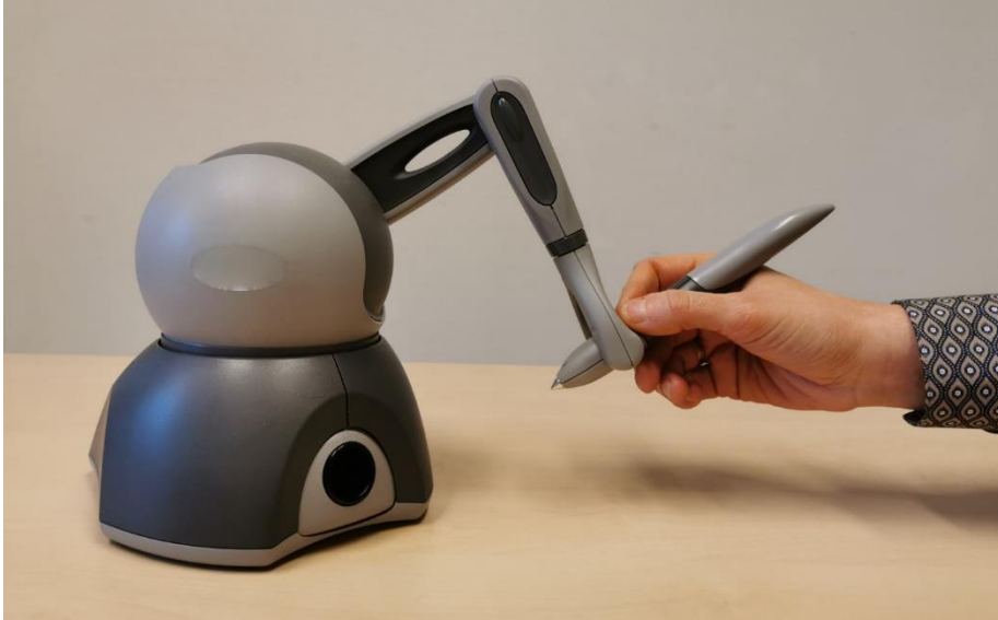
Figure 5. Phantom Omni haptic device was used in the studies included in this thesis
