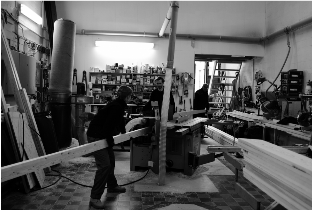
Wood planing and dimensioning at a local carpenter
