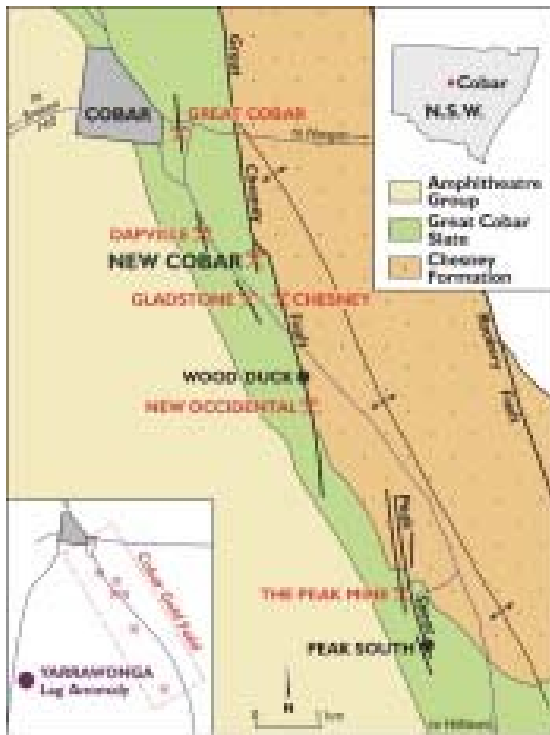
Figure 1. Cobar Basin location and setting. The Cobar Basin is situated in central New South Wales, Australia. It hosts steeply west dipping strata ranging from late Silurian to early Devonian in age. Ore deposits are found primarily in the Great Cobar Slate and Amphi theatre Group.
