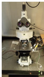
Figure 11. Ex-vivo physiology; whole cell recordings Brain regions are identified using a 10x/0.30 objective attached to a Nikon FN-1 microscope. Medium spiny neurons (MSN) are localized using a 40x/0.80 water immersion objective. MSN are voltage clamped at -70 mV.
