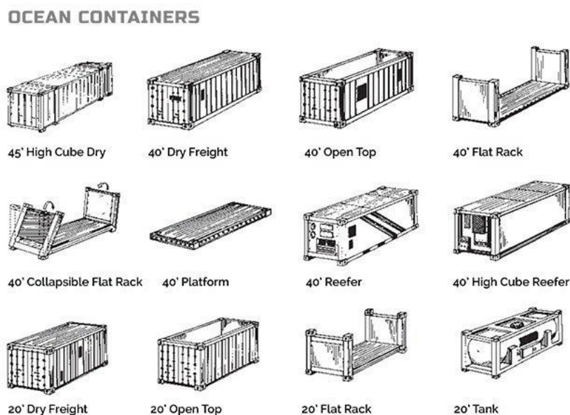
Figure 1: Illustration of different ISO container types (Croome, 2017)
