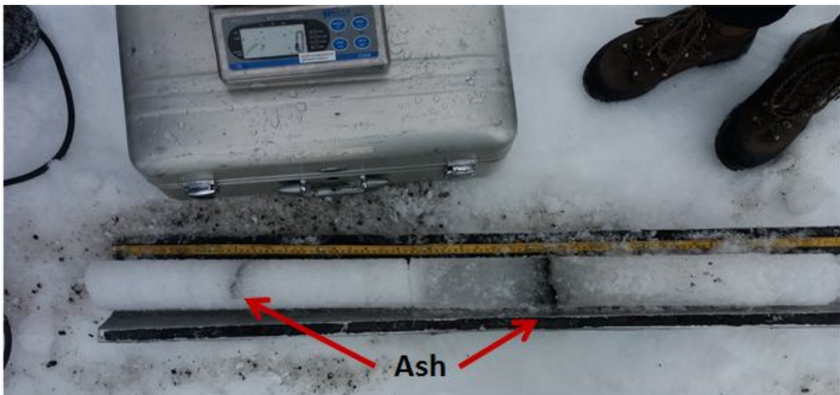
Figure 1.4: Labeled photograph of the 2019 ice core in June in the Grímsvötn caldera, showing layers of ash. Photograph courtesy of Pálsson (2020).
