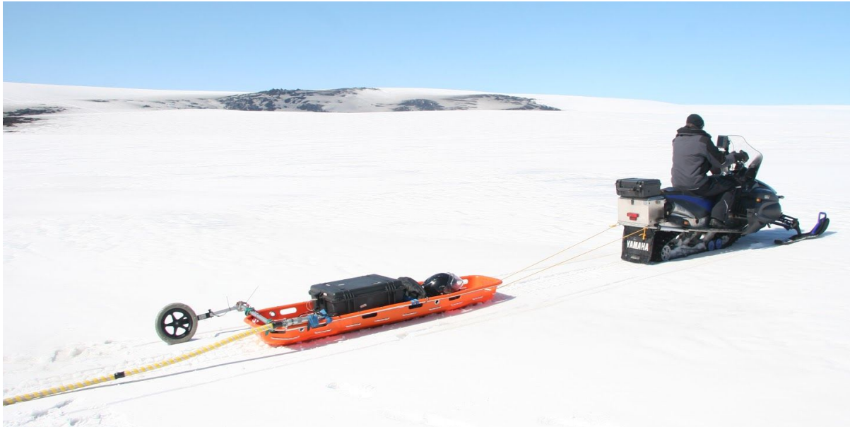
Figure 2.2: GPR setup from summer 2019 with RTA antenna (yellow cord) and measuring wheel coupled to a sled behind a snowmobile. Photo courtesy of Professor Erik Sturkell & Jon Kjartansson (2020).
