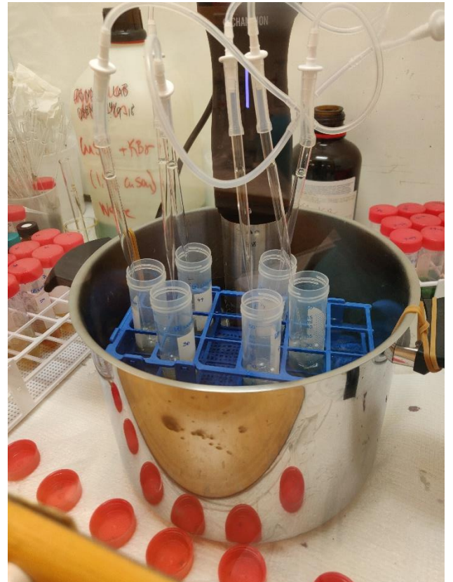
Figure 12. The DCM being evaporated from the soil, leaving the
