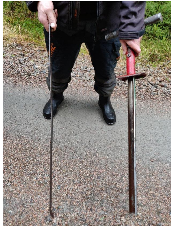
Figure 4. The soil sampler, with its two different parts.
