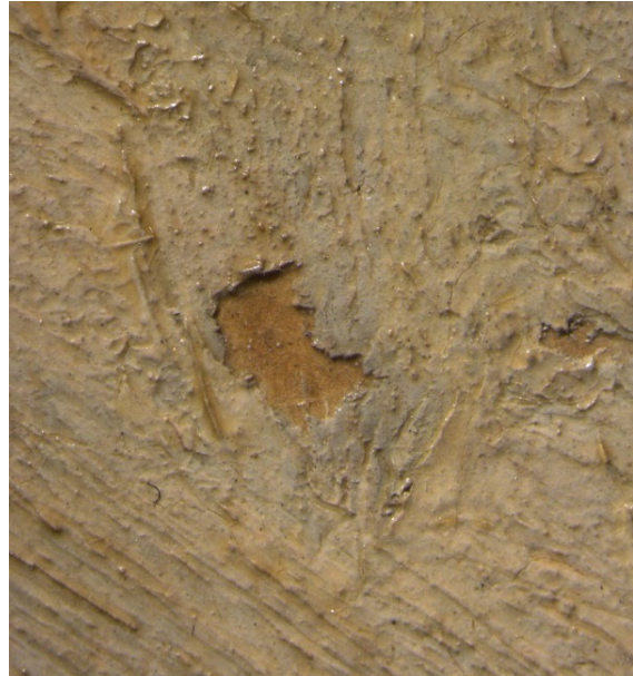
Fig. 22. Macro image (magnification 7.5x) of area with pigment loss, where the paint appears to be chipped off. Varnish seems to be present even in area of loss.
