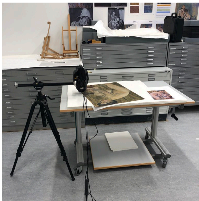
Fig. 14. Setup for XRF spectroscopy of WL84 at GMA.
