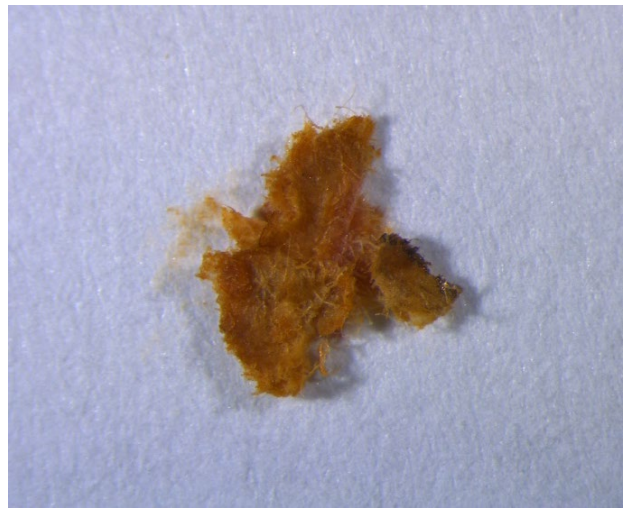
Fig. 60b. Cardboard sample after acidity test. A yellow color has developed, indicating acidity.
