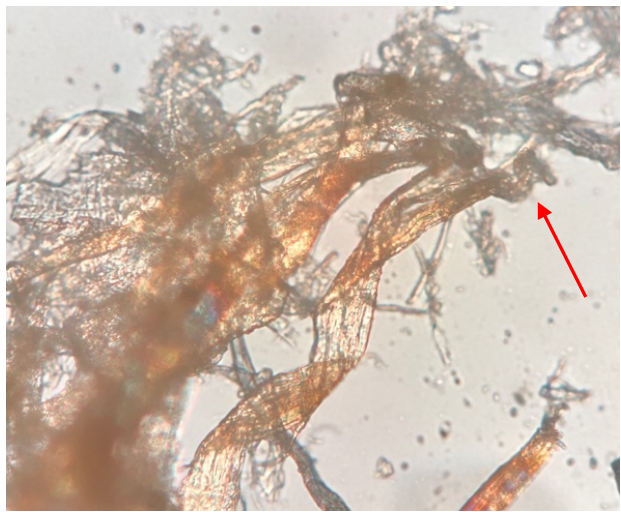
Fig. 55. Macro image (magnification 63x) of fiber with characteristic ribbon-like twists of cotton. A tapering tip can also be seen at the end of the fiber (marked with red arrow).
