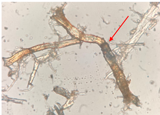
Fig. 57. Macro image (magnification 63x) of fiber with 'knees' or 'joints' (marked with red arrow), indicative of bast fibers.
