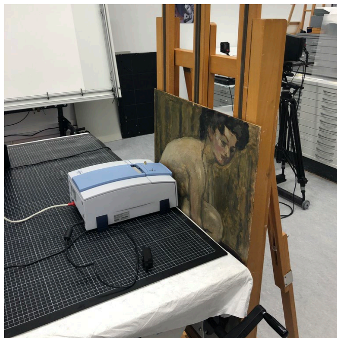
Fig. 15. Setup for FTIR spectroscopy of WL84 at GMA.
