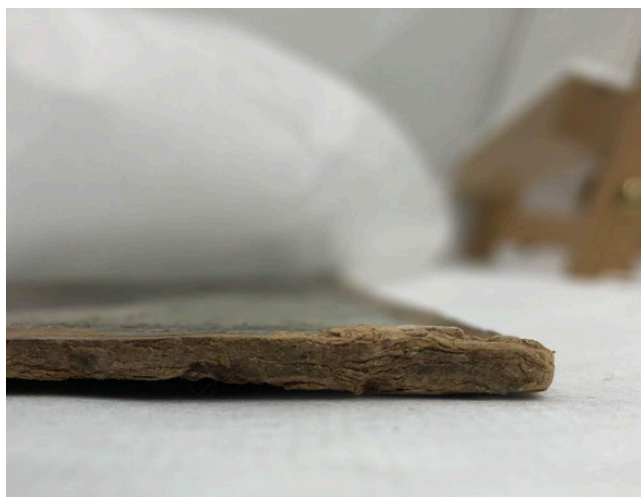
Fig. 37. Detail image of a corner of the cardboard, where there is slight delamination.
