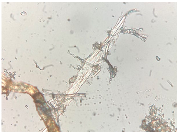
Fig. 56. Macro image (magnification 63x) of fiber that is twisted and has the appearance of a collapsed tube, indicative of cotton.
