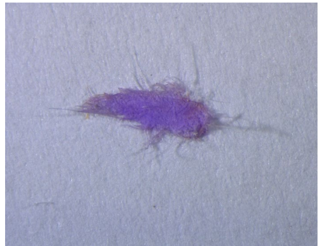
Fig. 59b. Control paper after acidity test. A strong purple color has occurred, indicating neutrality or alkalinity.
