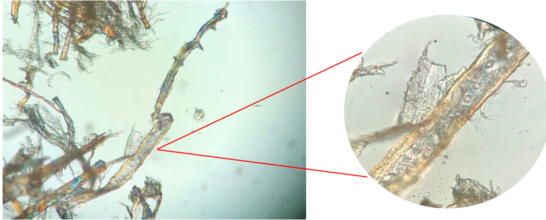
Fig. 53. Macro image (magnification 20x) of fiber with pits, shown in close up image (magnification 63x), indicative of wood fiber.
