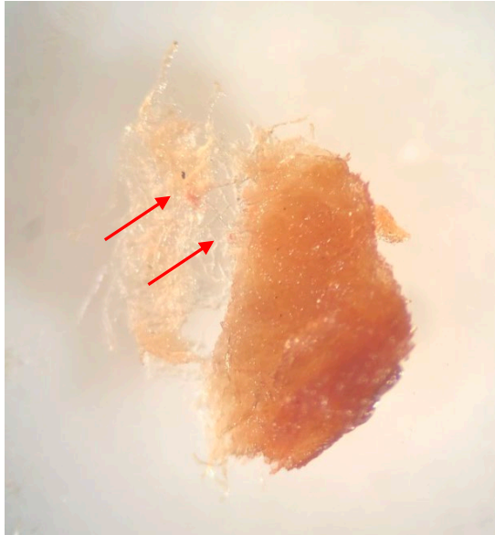
Fig. 58. Macro image (magnification 3.5x) of cardboard sample after Phloroglucinol spot test. Magenta areas are marked with red arrows.
