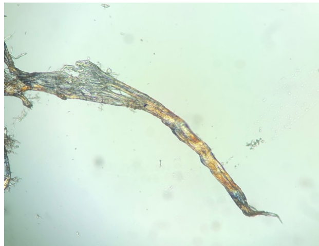
Fig. 52. Macro image (magnification 20x) of fiber with choppy, macerated end. Most likely woodpulp fiber.
