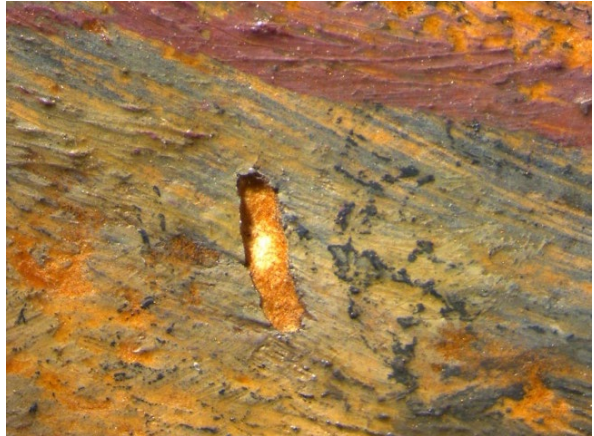
Fig. 26. Macro image (magnification 7.5x) of dent in cardboard and paint layer.
