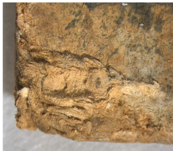
Fig. 38. Macro image (magnification 7.5x) of lower left corner of the cardboard, where the paper layers are abraded.
