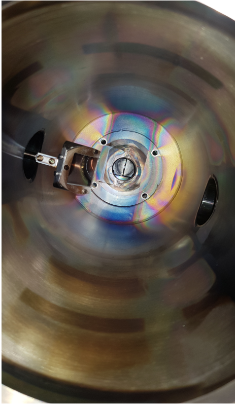
Figure 46: X-slit and mirror to monitor ionizer glow
