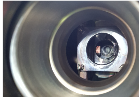
Figure 12: Picture looking into the beamline from the position of the ion source. Starting with cylindrical electrodes of the einzel lens, flat electrodes of the x-lens and the x-slit.
