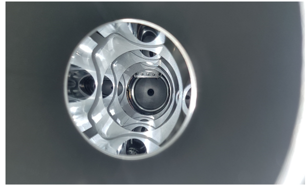
Figure 16: Picture looking into the beam line through the exit of the quadrupole triplet lens
