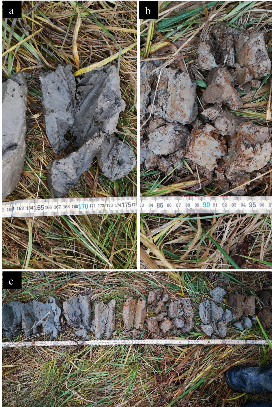
Figure 19. The sub-sample from site H19031 that had a pH-value of 3,13 after oxidation can be seen in picture a. The rust precipitates can be seen in picture b, and a part of the horizon can be seen in picture c.
