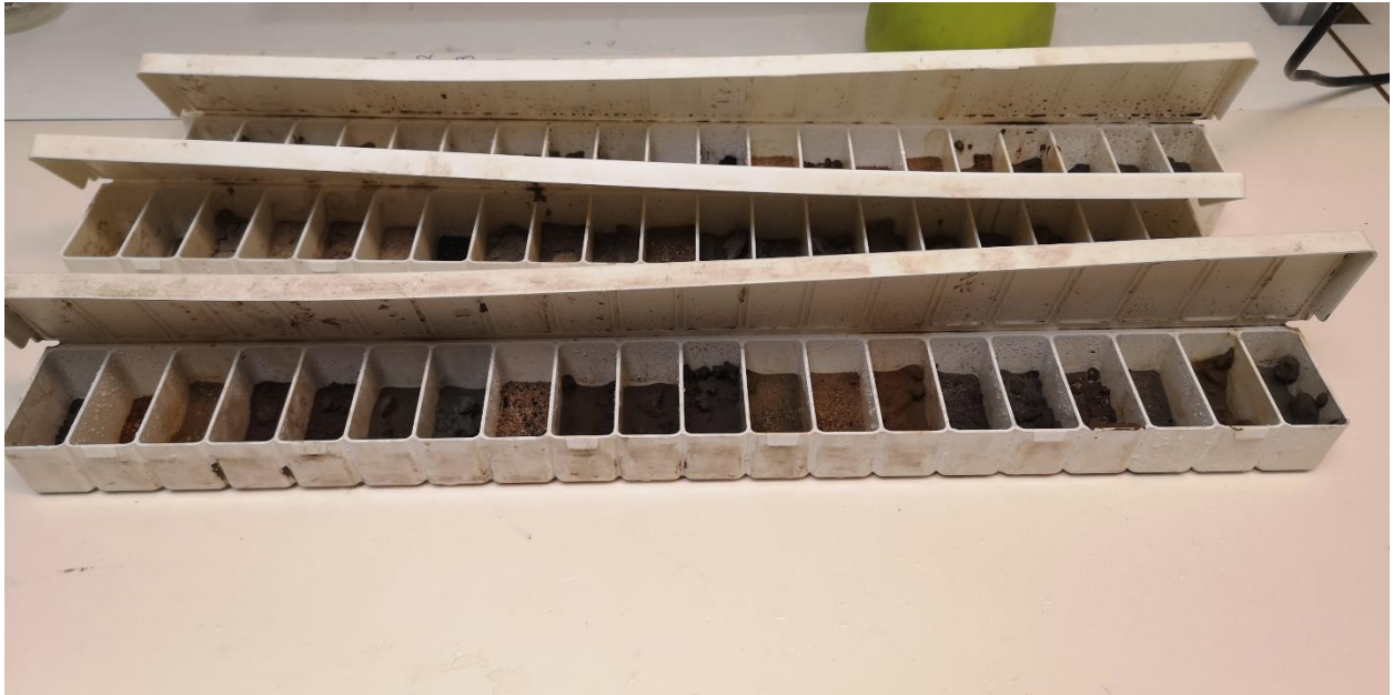
Figure. 8. The chip trays in which the soil samples were stored and oxidized. The soil samples were sprayed with deionized water to keep them under field capacity during the 9 weeks oxidation time.
