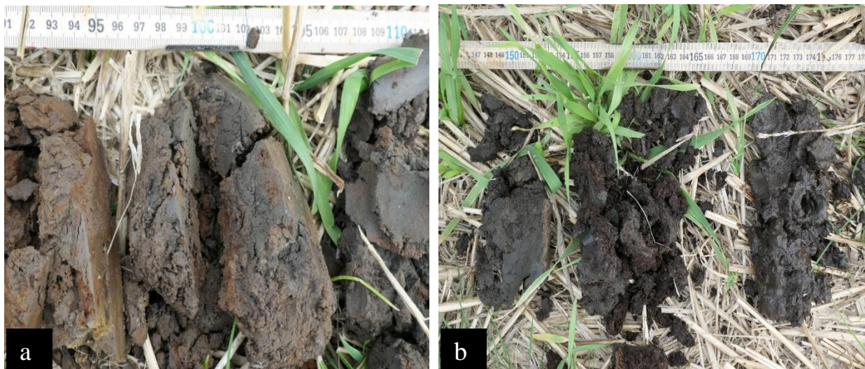
Figure 16. Pictures from site H19001 where the active AS soil layer can be seen in the top picture (a), and the peat layer can be seen in the bottom picture (b). Photo: Christian Öhrling, SGU.
