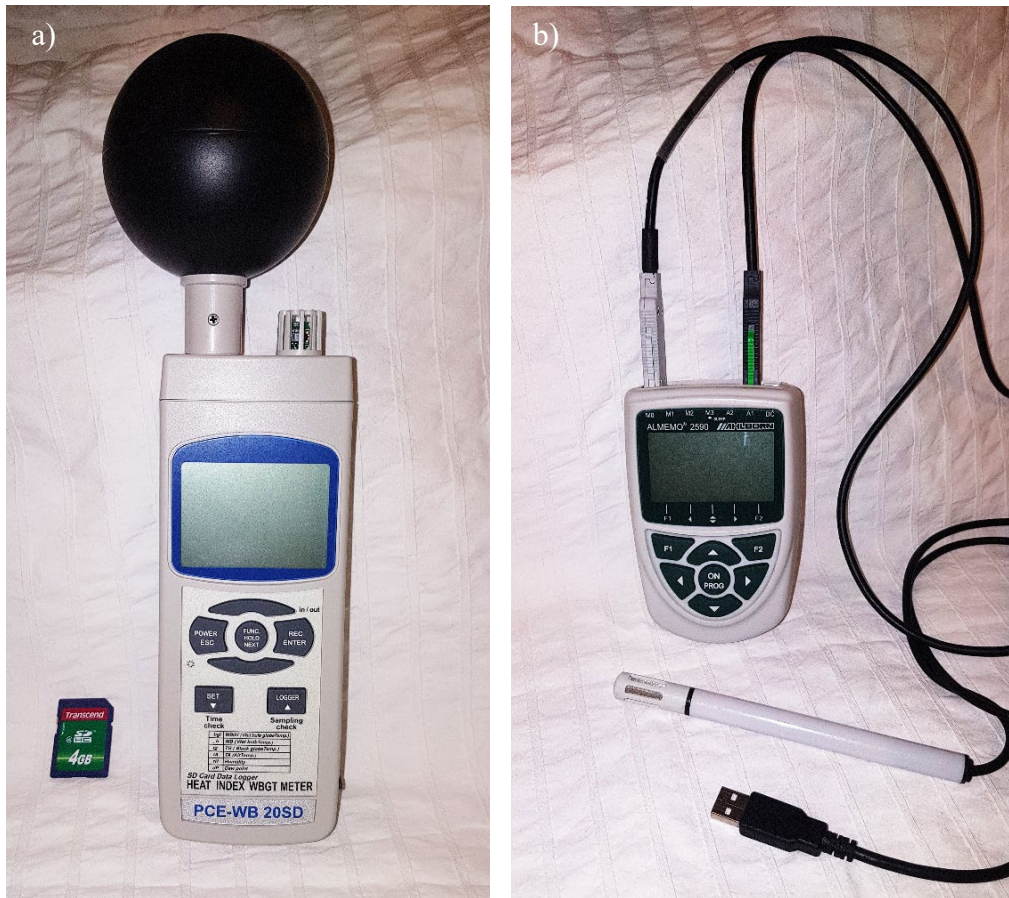
Figure 1: a) PCE-WB 20SD WBGT monitor with its 75mm black brass ball (left) and air temperature and humidity sensor (right), SD-card for data extraction next to the monitor. b) ALMEMO® 2590-2A/-4AS data logger connected to the combined capacitive air temperature and humidity sensor (FHA646-E1)(grey connector) and a USB connector to extract data (black connector).
