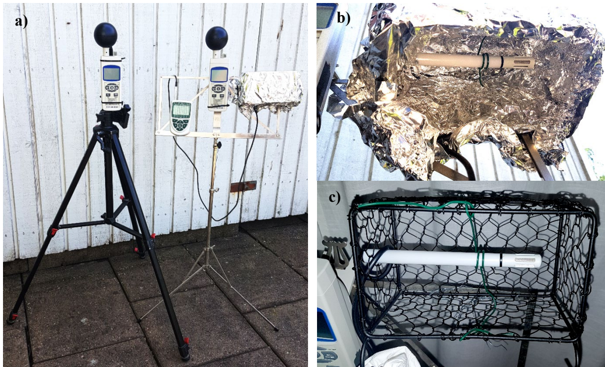
Figure 2: a) Improvised measuring stands composed of an old camera tripod (instrument 1 during experiments) and a note stand (instrument 2 during experiments), b) radiation shield composed of aluminium foil, and c) frame of the radiation shield.
