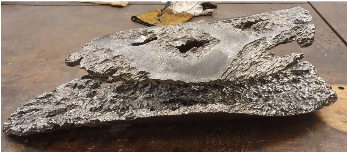
Figure 27. Texturing done and the two halves welded together, Halkosaari, 2020
