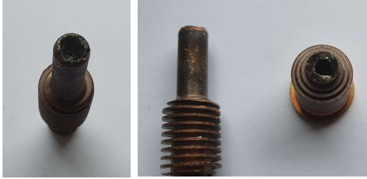
Figures 8a, 8b. Worn out and unusable electrode and nozzle. Halkosaari, 2020
