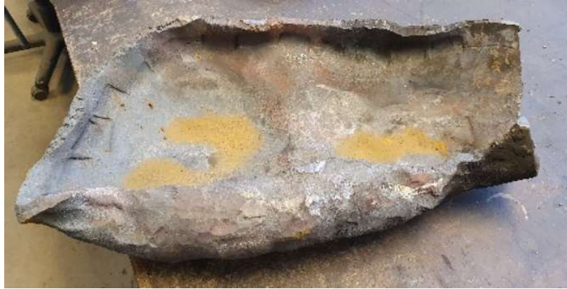
Figure 45. Roughly forged bottom half, Halkosaari, 2020
