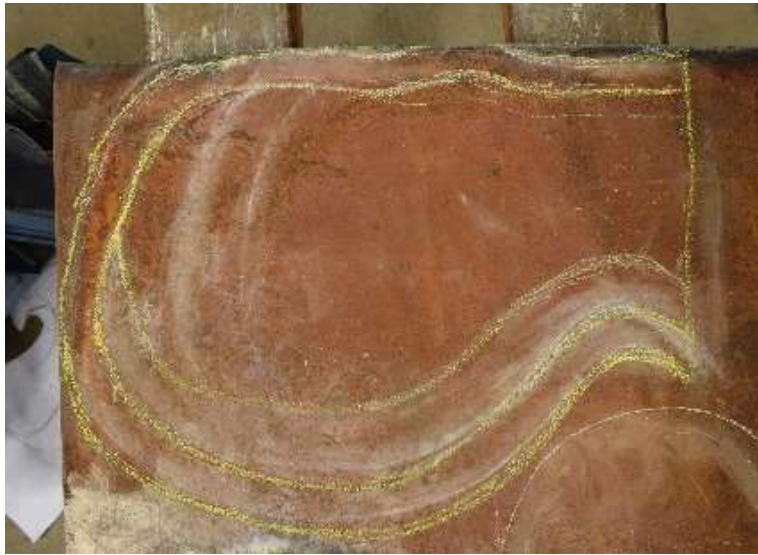
Figure 43. Template of the bottom half, Halkosaari, 2020
