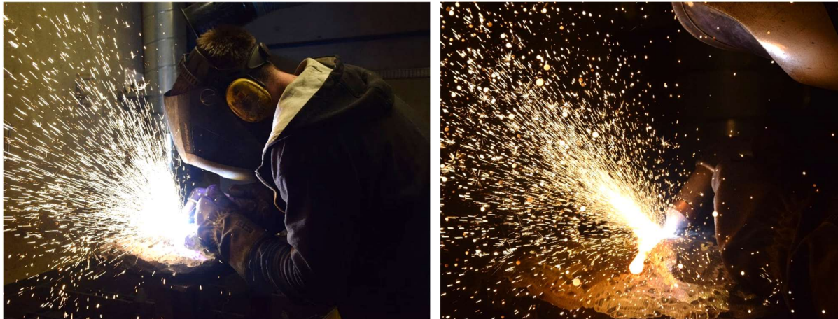
Figures 10a, 10b. Halkosaari, Postlmayr, 2020 Left: Plasma cutting in process. Right: Close up. You can see the slag starting to puddle up.
