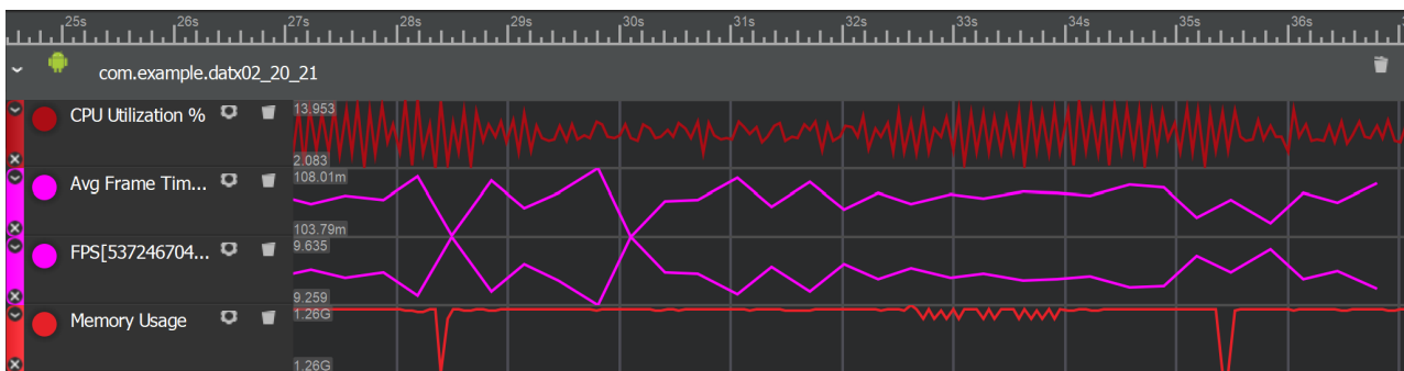
Figure A.12: Snapdragon Profiler graph with a grid size of 72x142x72, measuring CPU utilization, time per frame, frames per second and memory usage
