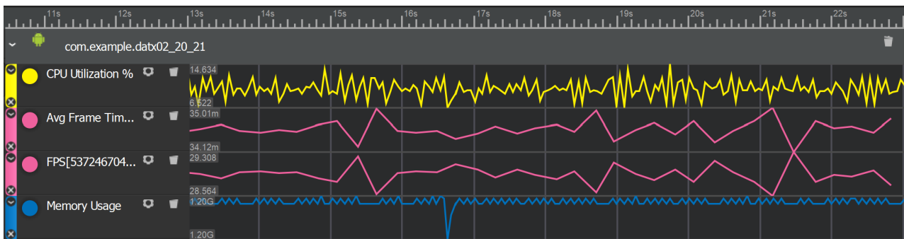
Figure A.18: Snapdragon Profiler graph with a grid size of 32 \times 122 \times 32 , measuring CPU utilization, time per frame, frames per second and memory usage
