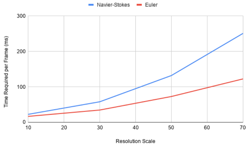
Figure 6.4: Graphing the performance of the Euler simulation approach and Navier-Stokes simulation approach in regards of time per frame when using a grid scale ratio of 1x4x1
