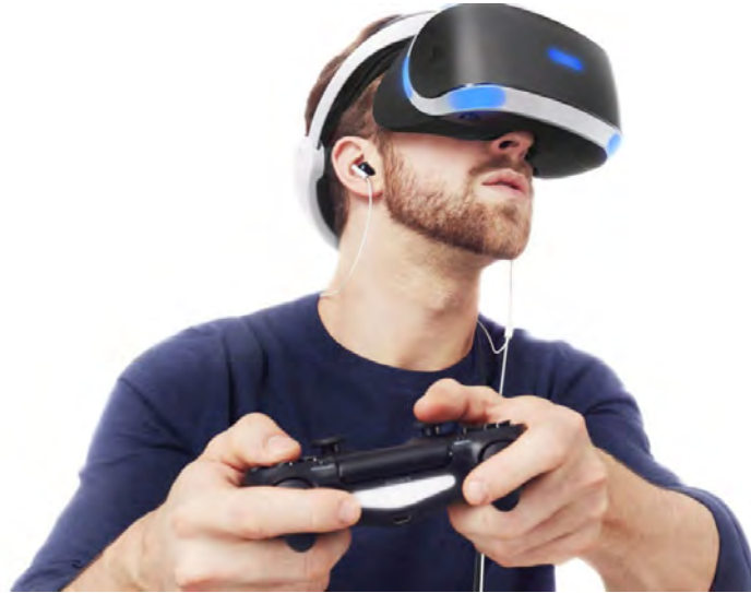
Figure 1.2: Playstation VR headset developed by Sony which can be played by plugging in the headset to the Playstation console.[2]
