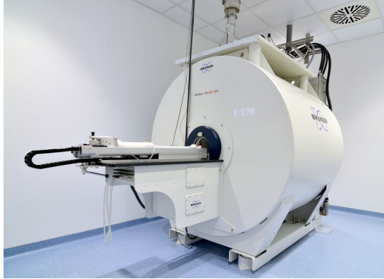
Figure 12. The 7T small-animal MRI system
