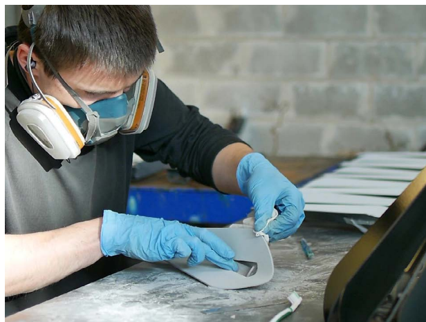
[fig.46.] removing the excess enamel from the edge
