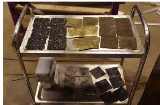
Left: 3 pcs, models in 1:10 scale, where the black ones are primed with wood glue, graphite powder, and clear coat. Right: material samples with blasting sand, plastic granules and graphite powder. Study of different surfaces.
