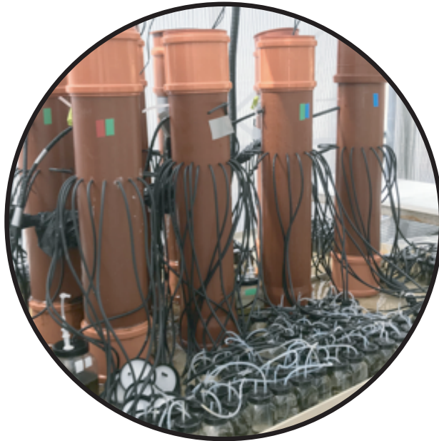
Figure 2. Experimental set-up of header tanks that can distribute experimentally controlled seawater with specific salinity, pCO 2 , and/or temperature as used in the greenhouse facility at Tjärnö Marine Laboratory.
