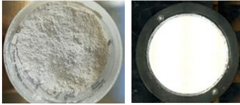
Fig. 4.5: Commercial lime hydrated in powder form from the company Finja (Murkalk 'Finja').
