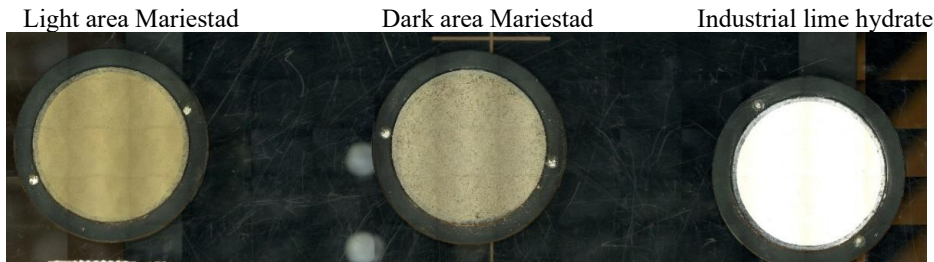
Fig. 4.1: The samples ready to be tested in the XRF and XRD. The samples were ground into a fine powder.
