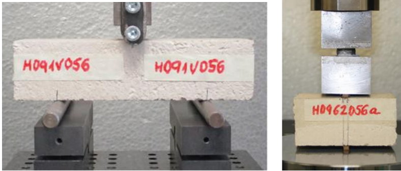
Fig 2.2. Three-point flexure test (left) and splitting test (right) (archive of Garijo et al. 2019).
