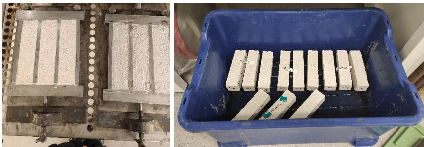
Fig. 4.13: The mortar in the forms and the ones with pozzolana stored over water.
