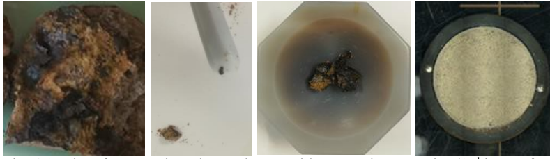
Fig. 4.3: Lime from Mariestad – Dark area with magnetic properties (2 nd image from left).
