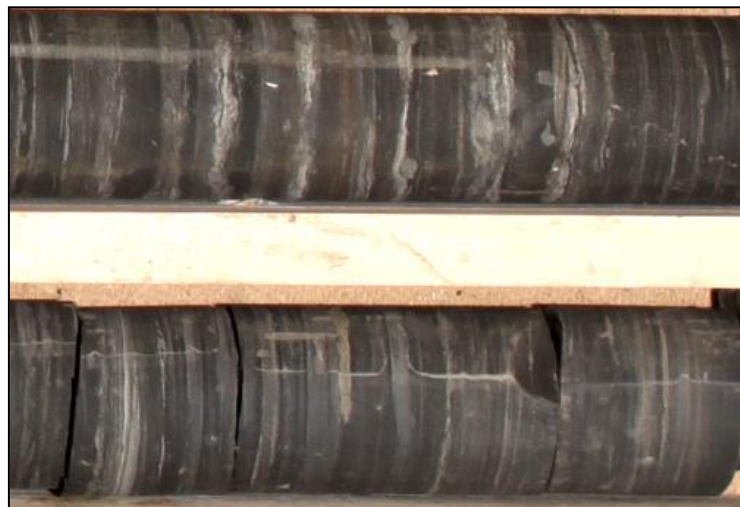
Fig. 23. Close up of lenticular bedding in core 13-2013, the upper core showing small burrows and sand lenses disturbed by bioturbation.
