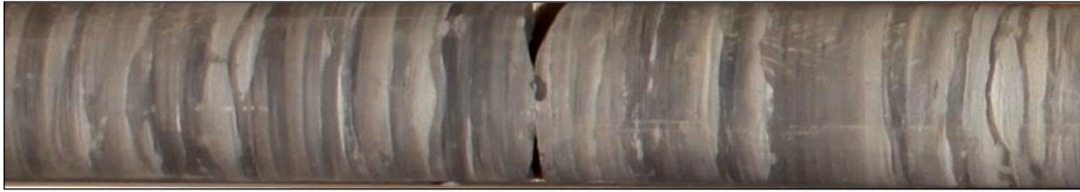
Fig. 24. Close up of wavy bedding in core 13-2013.
