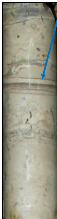
Fig. 18. Facies 2, light coloured paleosol beneath a thin coal seam in core BH-15-2010. The figure to the left shows a closeup of structures and rootlets.
