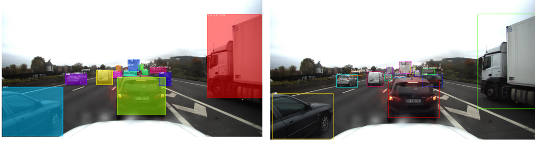
Figure 4.2: Visualized results of Mask R-CNN to Volvo's dataset: On the left, is the actual annotated image and on the right, is the predicted objects from our model.
