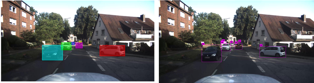
Figure 4.4: Visualized results of YOLOv4 to Volvo’s dataset: On the left, is the actual annotated image and on the right, is the predicted objects from YOLOv4 model
