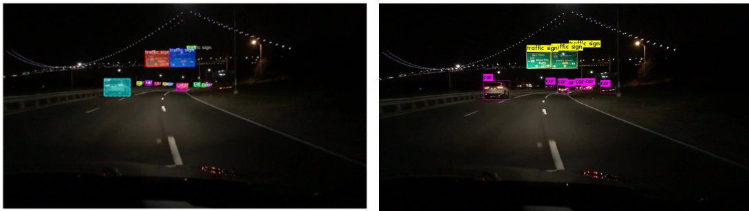
Figure 4.3: Visualized results of YOLOv4 model: On the left, is the actual annotated boxes and on the right, is the predicted objects from YOLOv4 model.
