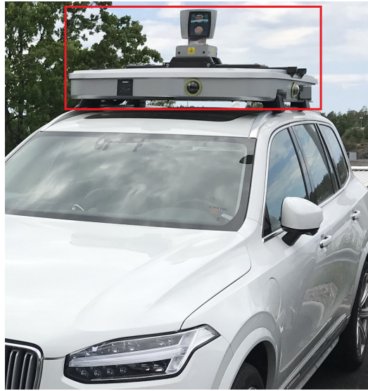
Figure 1.1: The reference box placed on the roof of the vehicle, which is used for the AD and ADAS development and verification.
