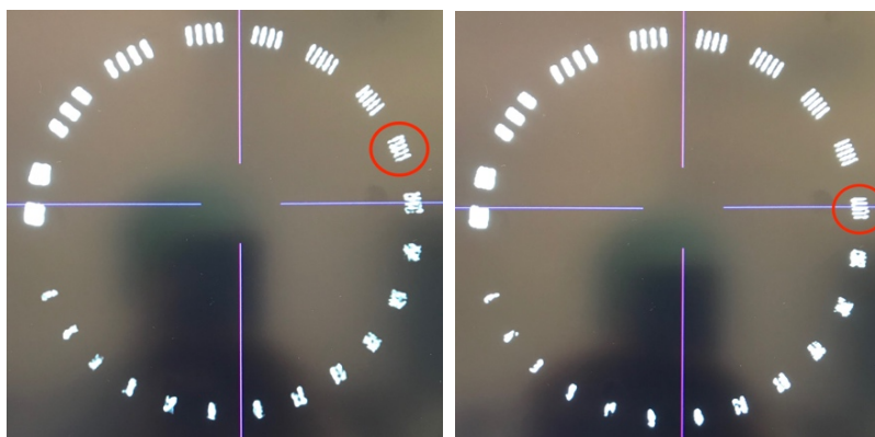
Figure 4.3: Schematic image of the number of line pairs per cm after a CBCT on Artis Q, Pheno and Zeego. The left figure represents 8 lp/cm and the right 9 lp/cm.
