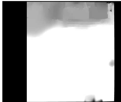
Figure 4.4: The filtered disparity map for Figure 4.3. A brighter value indicates a higher disparity value.
