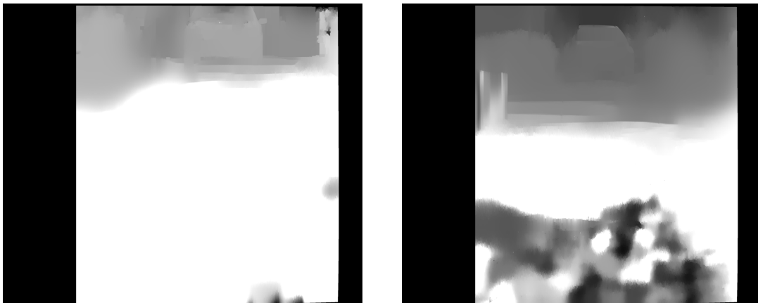
Figure 3.15: The filtered disparity maps for Figure 3.8. A brighter value encodes a higher pixel disparity.
