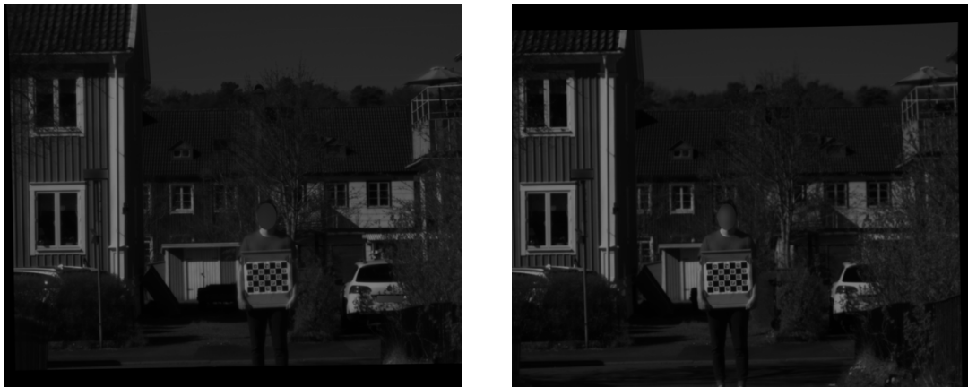
Figure 3.4: The images from Figure 3.3 after applying the rectification.
