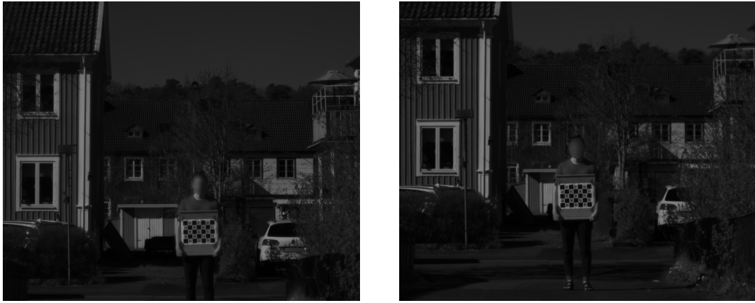
Figure 3.3: Example images for the stereo calibration, with the chessboard present.
