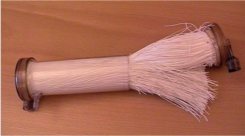
Figure 7. A dialyser tube divided to show the amount of fibres. With kind permission.
