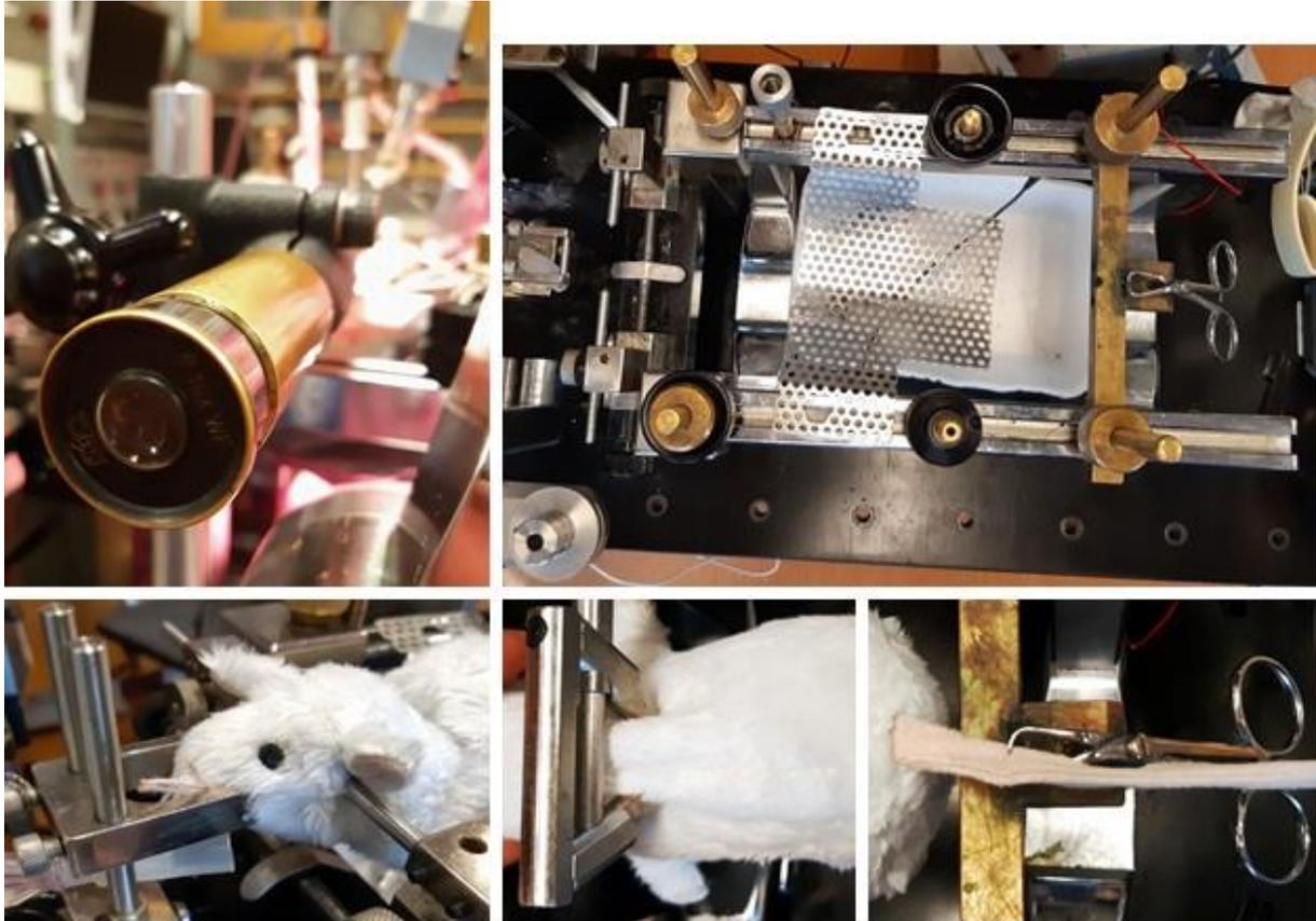
**Figure 8:** Spotting scope for final alignment of electrode tips (A). Metal frame, carefully electrically grounded, to which the preparation is secured (B). Plush toy rat demonstrating fixation of the head (C), spinal column (D) and tail (E) to the metal frame.
