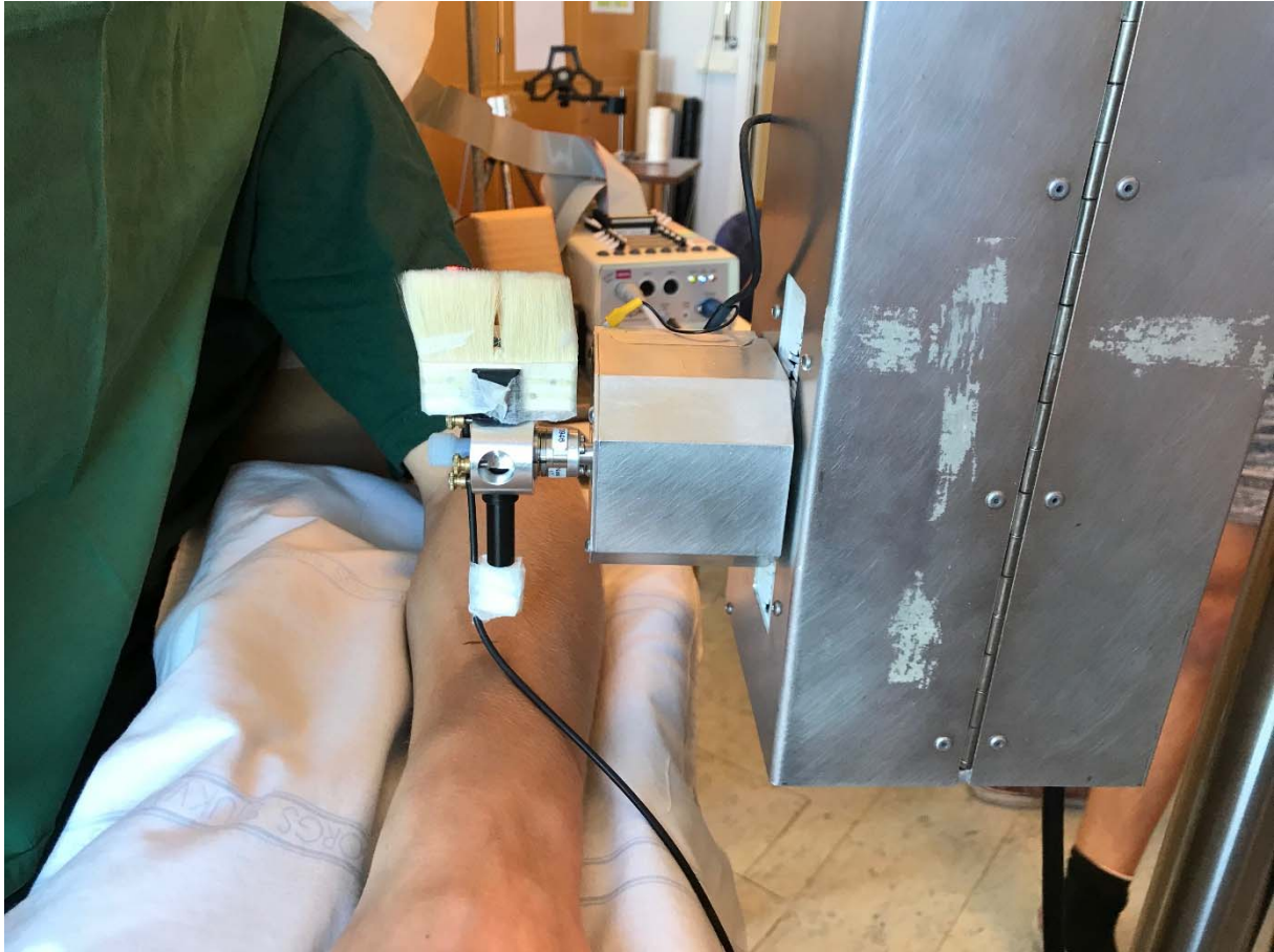
Figure 2. A participant's left arm fixated on the vacuum pillow. The RTS brush is seen in standby mode with the brush pointing up. The optical sensor is barely visible at the top.
