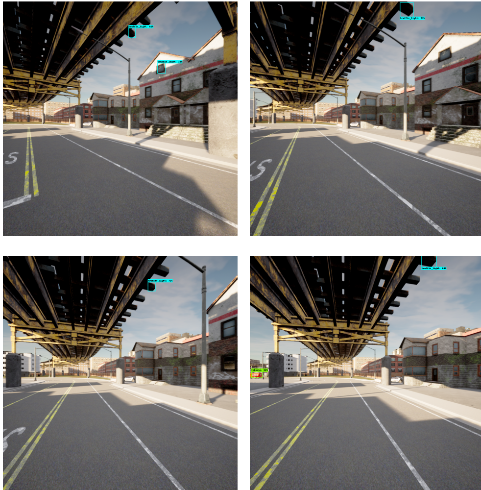
Figure 3: A traffic light incorrectly detected during several consecutive frames
