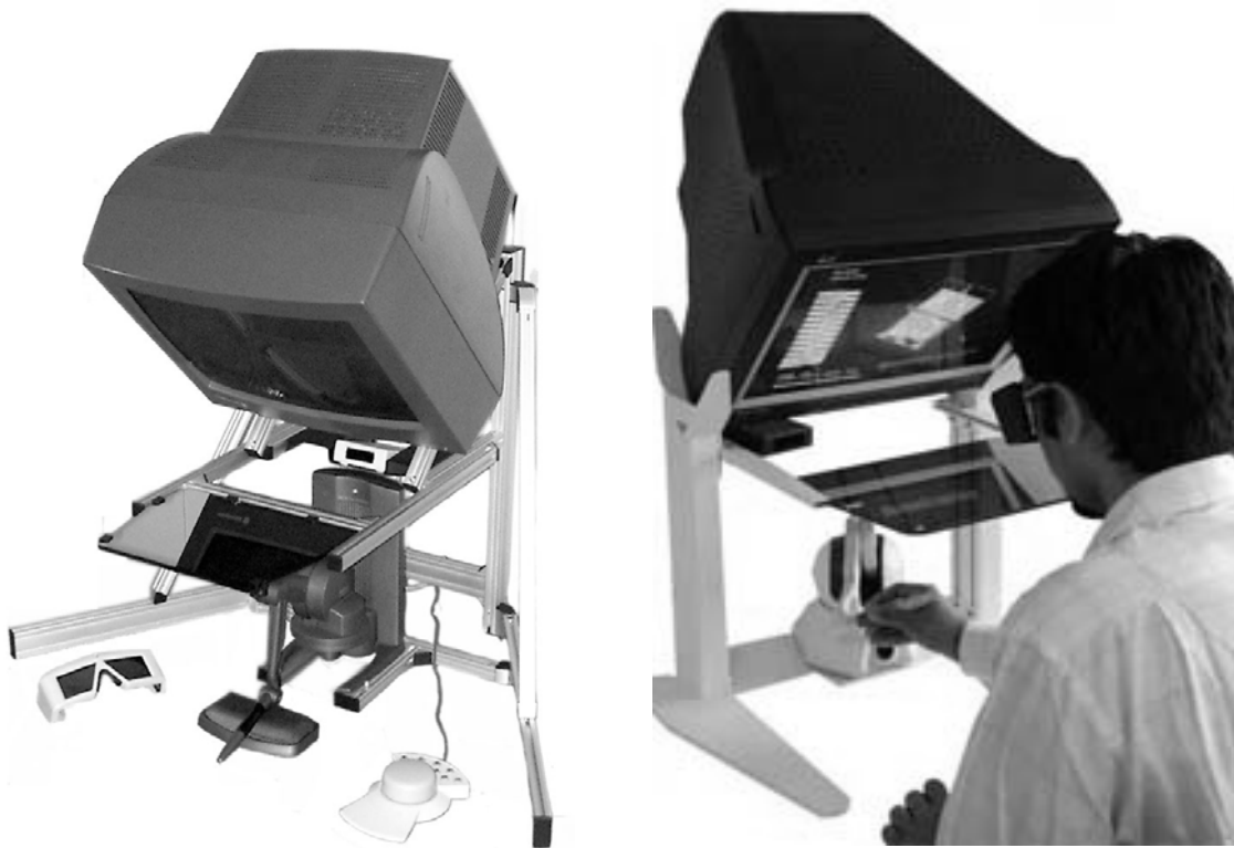
Figure 2. Semi immersive workbenches, Reachin (left) and Sensegraphics (right). Pictures reproduced from 3Dcgi.com and Sensegraphics AB.
