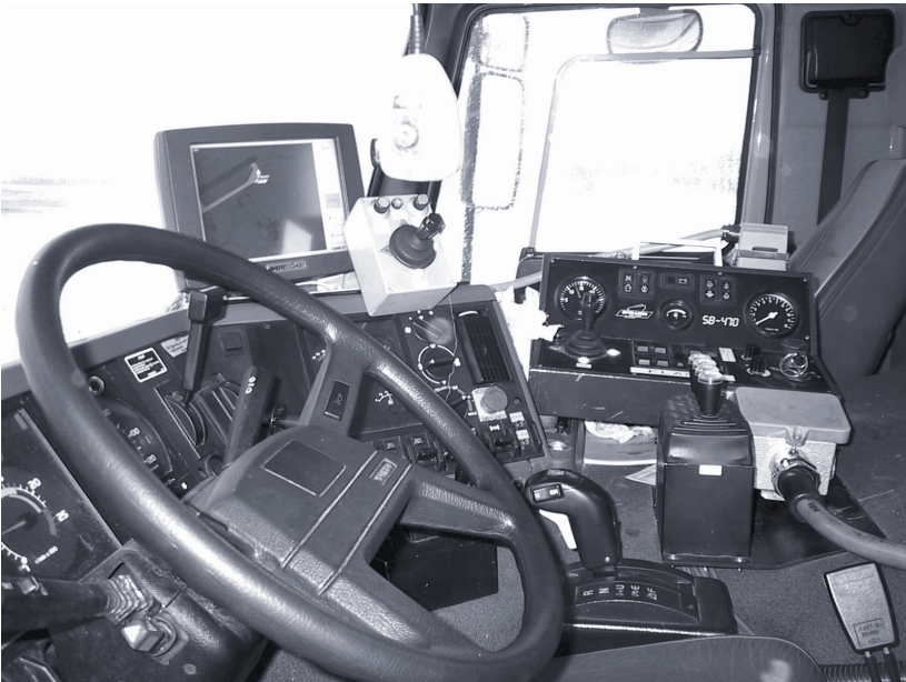
The inside of one of the snow vehicles. The SnowCard display is in the upper left corner of the picture. The small radio receiver is hanging down from the ceiling of the vehicle, and is visible in the top middle of the picture.
