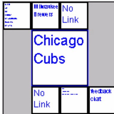
Fig. 4. The Web browser of Small Terminals (WEST). All three views are shown in their actual resolution of 160*160 pixels. The views are, from left to right, the thumbnail view, the keyword view and the link view.
