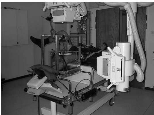
Figure 10. The RSA lab with two ceiling-mounted radiographic tubes (© Knee Surg Sports Traumatol Arthrosc)
